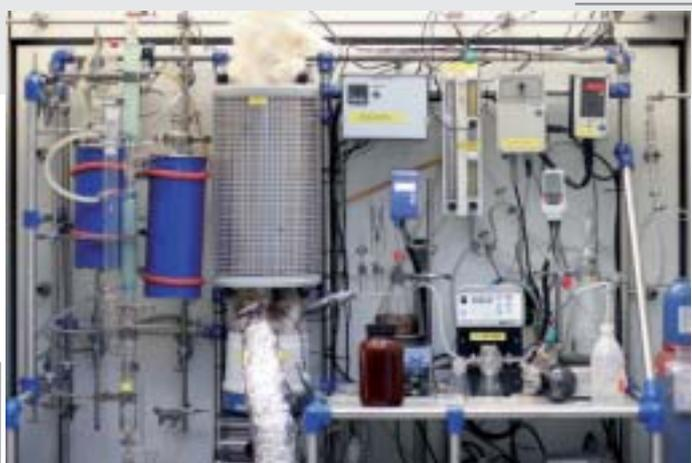
The use of silica or alumina-based catalysts is known for the catalytic conversion of biogenous fats and greases to long-chain hydrocarbons and simple aromatic compounds. The utilization of activated carbon as catalyst with simultaneous steam addition represents a promising alternative.
