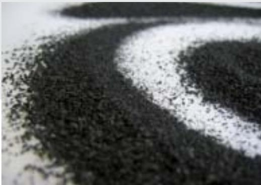
Plastic powder for coatings and laser sintering processes
